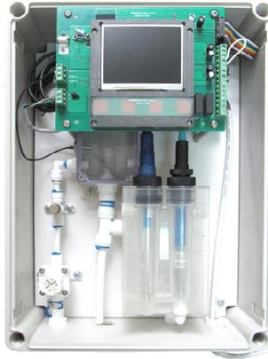
Figure 3. Integrated Free Chlorine /CLO<sub>2</sub>/pH Online Analyzer inside
